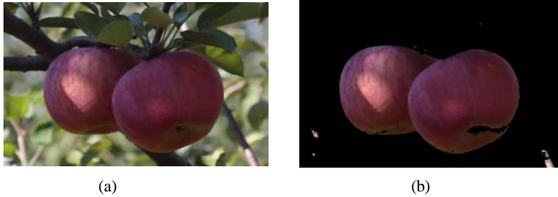
Fig. 2. Example of the result of K-means clustering segmentation: (a) the re-sized original image, (b) the segmented image by using improved K-means clustering algorithm.
