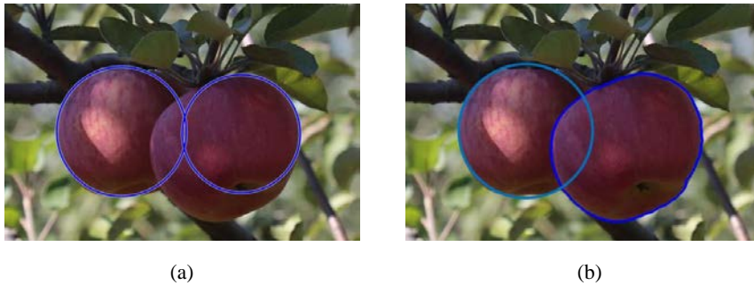
Fig. 8. Results of comparison between CHT method and proposed method: (a) result of detection of overlapped apples with CHT method, (b) result of detection of overlapped apples with proposed method.
