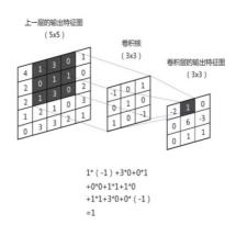
Fig.2 Schematic diagram of convolution operation
