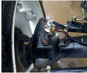
Fig.4 Fixed angle sensor
