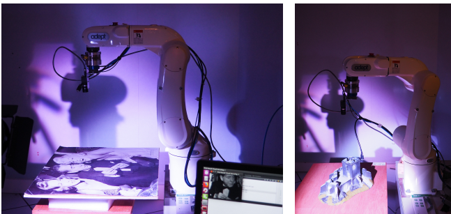
Figure 1. Experimental setup: camera mounted on a Viper 850 from ADEPT and the two considered scenes
