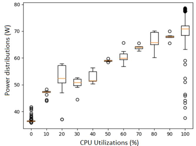
Figure 1. Distribution of power under different CPU-utilization.
