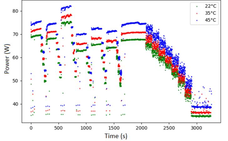
Figure 3. Server power under three different ambient temperatures.
