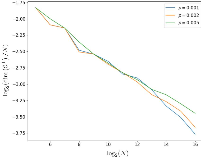
**Figure 2:** Log-log plot of rate  $\dim(\mathcal{C}^\perp)/N$  of the dual code vs the block-size  $N$  for binary symmetric channels at transition probabilities  $10^{-3}$ ,  $2 \times 10^{-3}$  and  $5 \times 10^{-3}$ .
