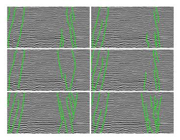
**Fig. 7.** From left to right and from up to down, the result of detection of the semblance coherence, the eigenstructure-based coherence, the variable scale semblance coherence, the variable scale eigenstructure-based coherence, the average of the two types of the variable scale seismic coherence and the LSE
