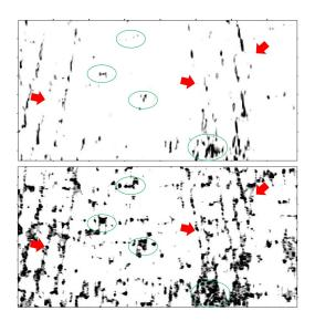
Fig. 3. The traditional eigenstructure-based coherence (above)and the variable scale eigenstructure-based coherence (below)
