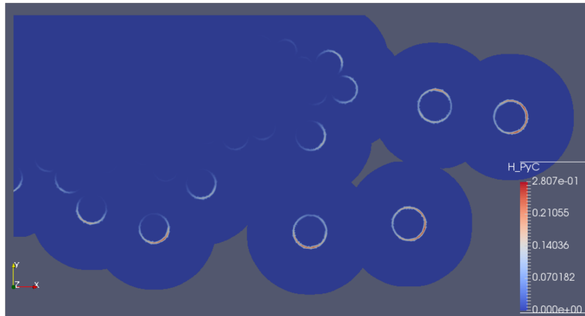
Figure 8: Consumed pyrocarbon height after 30 minutes.
