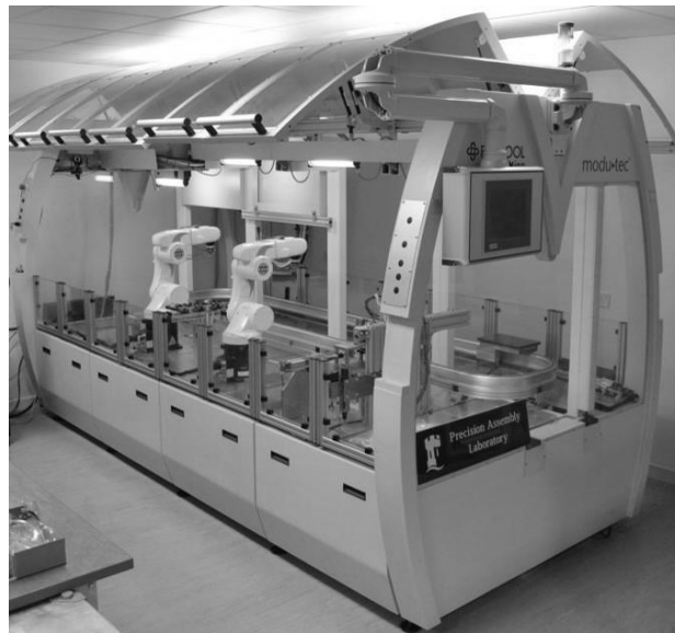
Fig. 3. The precision assembly demonstrator (PAD)
