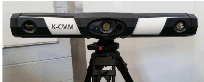
Fig. 5. K-CMM camera of the FA 3 D
