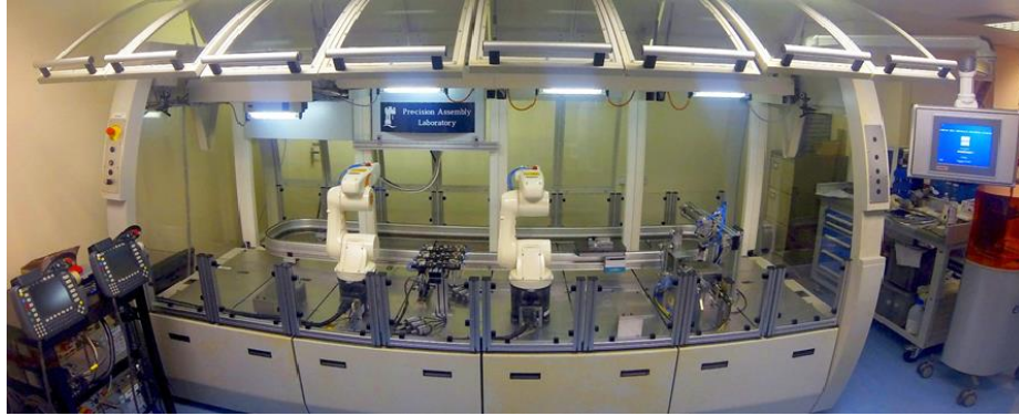
Fig. 3. The PAD assembly system [18] comprising two KUKA six-axis robotic arms with corresponding workspaces, a shared tool changing rack, a testing station, and a shuttle transport system, which links the stations to each other and a loading/unloading station.
