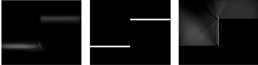
Fig. 3. Left: measured CSI interferogram. Centre: finite element model from CSI interferogram. Right: second-order CSI interferogram, clearly showing the vertical sidewall Coupland and Lobero 2009).
