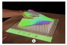
Fig. 21: (a) The EMERGE shape display featuring 10 by 10 bars [152]; (b) The inFORM shape display featuring 30 by 30 bars [41].
