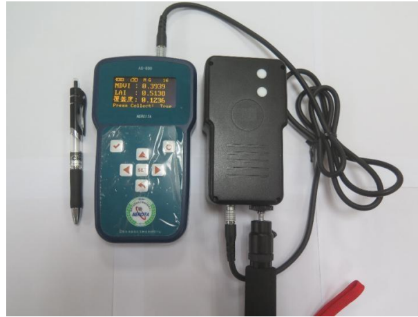
Fig. 3Instrument for measuring crop growth parameters
