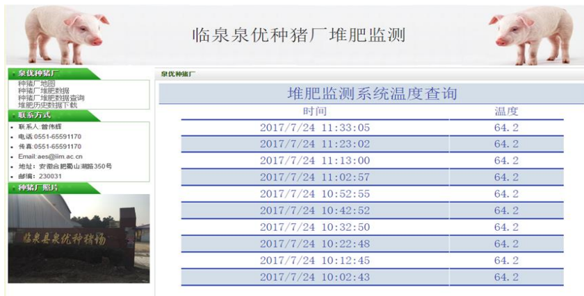
Fig. 6. The compost temperature monitoring platform web page
