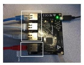
Fig. 11: The Zodiac Fx switch set-up.
