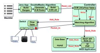
Fig. 10: Architecture and set-up of our SDN network.
