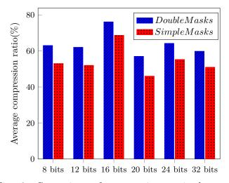
Fig. 9: Comparison of compressions ratio between *DoubleMasks* and *SimpleMasks* while varying the length of a field.
