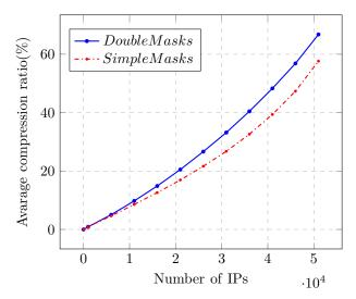
Fig. 8: Compression ratio of *DoubleMasks* and *SimpleMasks* using a synthetic dataset of range fields of length 16bits.
