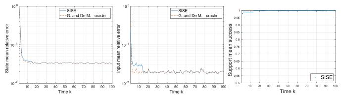
Fig. 2: Experiment 2: p = 40, m = 30, n = 50. The benchmark is an oracle version of [5] which knows the correct support. With m = 30, SISE achieves a perfect support estimation.
