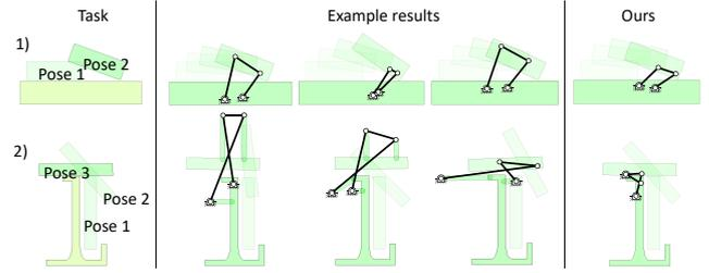
**Figure 17: User study.** The subjects were asked to do two tasks, 1) easy and 2) difficult ones. While most of the subjects could successfully find a valid solution that does not cause any collision from the first pose to the last pose, there is a significant error in the trajectory. Please see the accompanying video for the actual motion of the designed mechanism.
