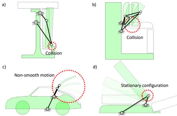
**Figure 15: The results by [MTG\*14].** The linkage synthesis approach of Megaro et al. [MTG\*14] does not consider any defect, collision, and the smoothness of the trajectory. As a result, the generated connectors may cause a-b) collisions, c) undesired trajectory, and d) some defects.
