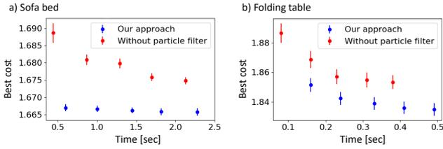
**Figure 14: Effect of particle filter optimization.** The blue points represent the best cost by our approach, whereas the red points represent the best cost obtained without particle filter optimization. For both, the points represent the mean values of 100 trials while the vertical bars show the 95% confidence interval.
