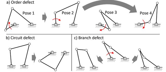
**Figure 6: Mechanism defects.** a) The linkage goes from the second pose to the last pose skipping the third pose. b) The linkage cannot go from the left to the right without disassembly. c) The linkage could go from the configuration in the middle to either the left or the right when rotating the driving link (red arrow).
