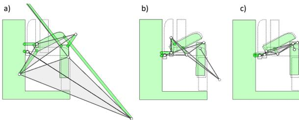
**Figure 11: Alternative solutions.** The user can interactively obtain different solutions by changing the weights for the soft-terms. a) When only accuracy is taken into account, the moving bodies traverse the input poses very accurately, but the linkage might become unnecessarily large. b) More smooth trajectory can be achieved by sacrificing the accuracy and size, while c) a smaller size of linkage can be achieved by sacrificing the accuracy and smoothness.
