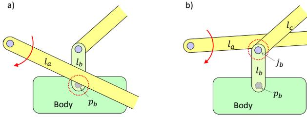
**Figure 8: Two cases of collision between links.** During the kinematic simulation, two types of collisions in 2D projected space are recorded: a) link  $l_a$  collides with  $p_b$ , the attachment point of joint connector  $l_b$ . b) link  $l_a$  collides with joint  $j_b$ .
