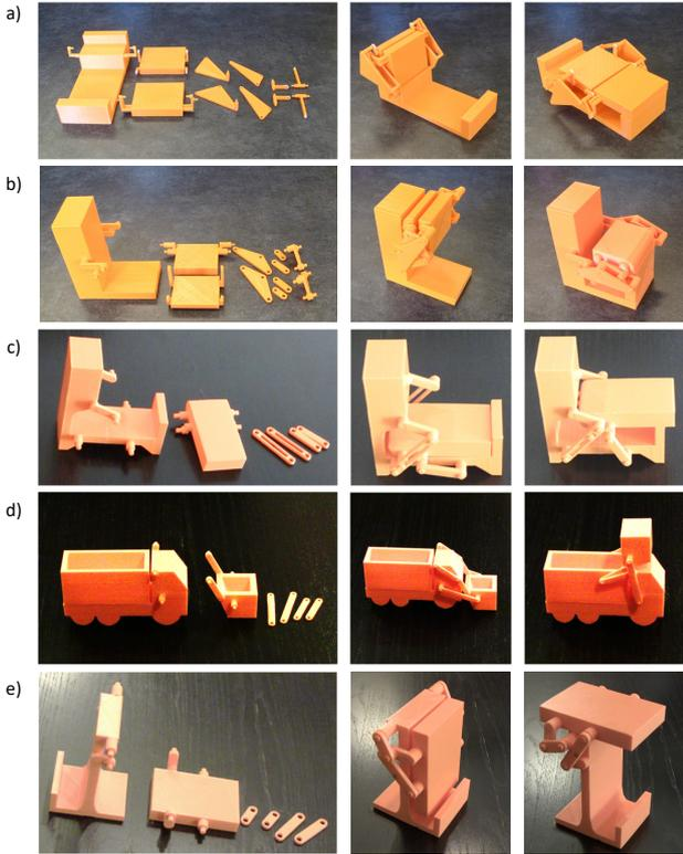
**Figure 12: 3D printed examples.** The output 3D geometry of a) wall bed, b) wall chair, c) sofa bed, d) garbage truck, and e) folding table were printed with a desktop 3D printer. The printed parts can be assembled readily without additional bolts and nuts.
