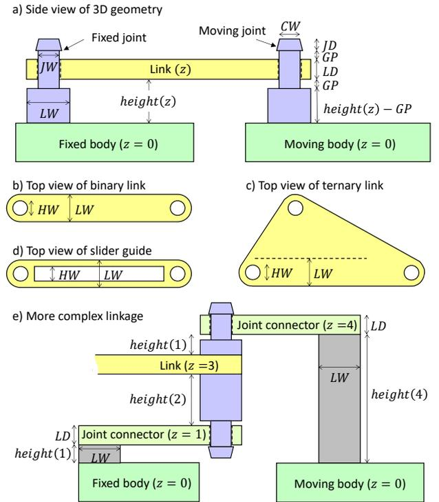
**Figure 9: Parameterized linkage geometry.** a) The height of the joints is computed from the depth of the link,  $z$ . b) Top view of a binary link. c) Top view of a ternary link. d) Top view of a slider guide. e) In the case where three links are connected via a joint, the joint should be attached to the link that is located in the middle, and other links have a hole at the corresponding position.
