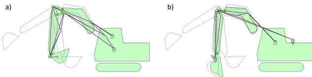
**Figure 16: Motion controllability.** Two poses may not be enough to achieve a desired motion. a) Using only two poses, the dipper shovel does not dig into the ground. b) Adding an intermediate pose allows the user to produce the proper motion.
