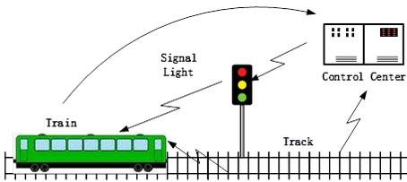
**Fig. 3.** Interlocking system
