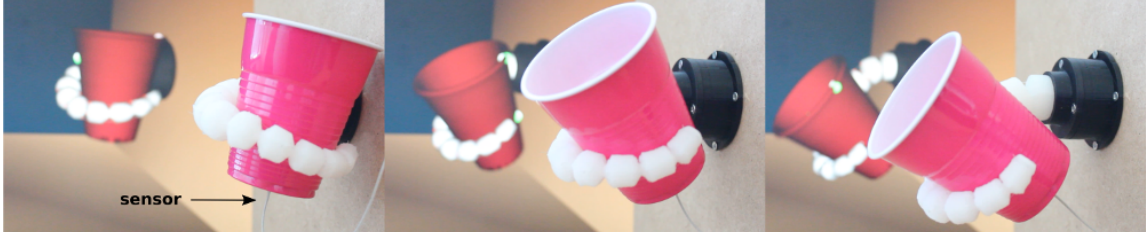
Fig. 9: Real soft robot actuated online using the output of the simulation. In this scenario, using our control framework, we are able to control the orientation of the real plastic cup (see the attached video).
