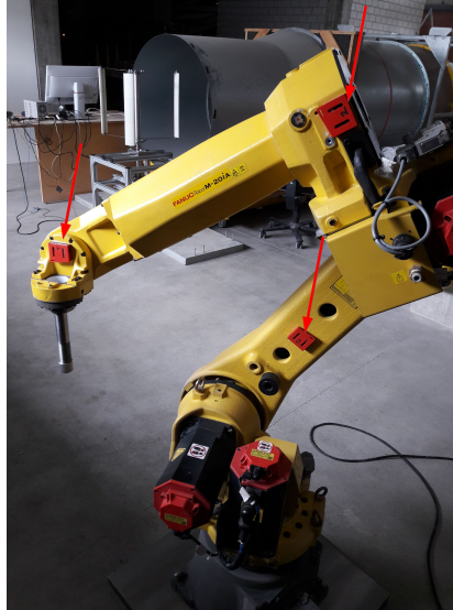
Figure 2: Installed base with mounted SensorTags
