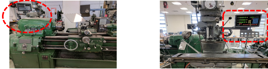
Figure 1. Smart Lathe (left) and Smart Mill (right) after DROs Installation
