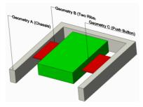
Fig. 2. Geometries that consist the push button.
