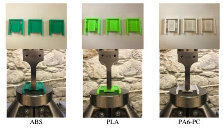
Fig. 7. Specimens and testing procedure.
