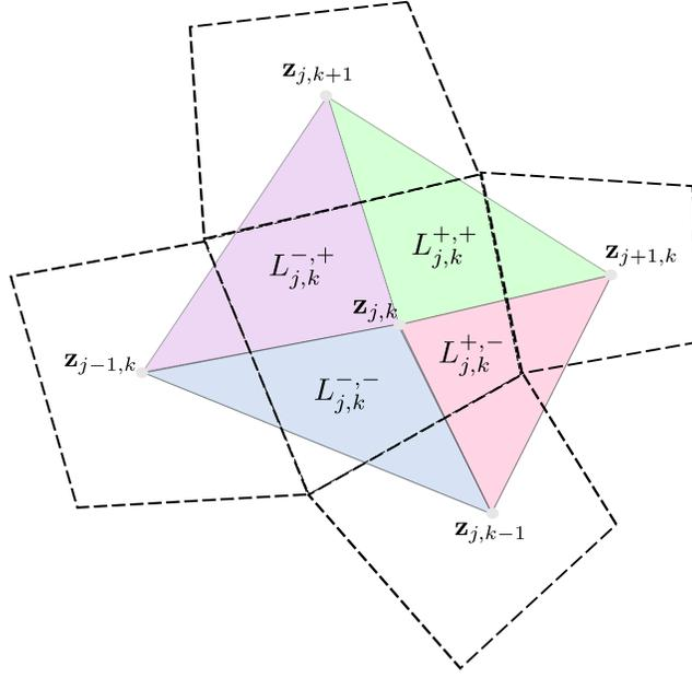
Figure 2.1: Four linear interpolants over cell  $I_{j,k}$ .
