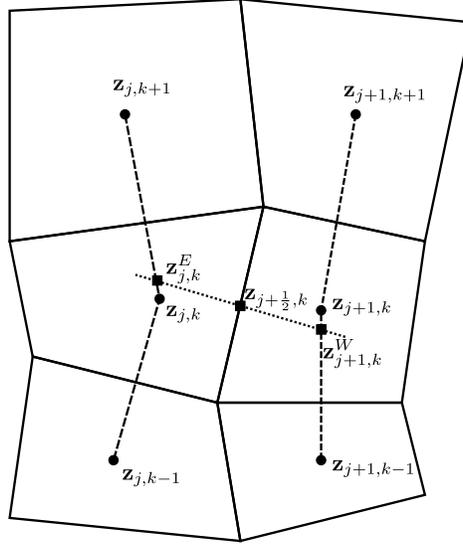
Figure 2.2: Set-up for numerical computations of normal derivatives.
