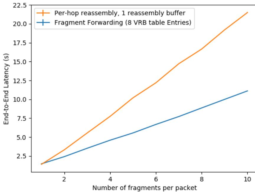
Figure 5: Comparing end-to-end latency with per-hop reassembly and fragment forwarding. Results are averaged over 100 simulation runs and plotted with a 95% confidence interval (which is too small to see in the plot). In this scenario, using fragment forwarding reduces end-to-end latency by roughly 50% when compared to per-hop reassembly.
