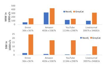
Figure 10: MIW and SIW benchmark throughput in 1,000 values/second. Bigger numbers mean better results. Numbers beneath dataset names mean number of nodes and edges, *i.e.* nodes x edges.
