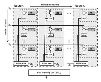
Fig. 1 Generic hardware architecture for a two-dimensional SOM.
