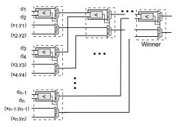
Fig. 2 BMU block diagram for a two-dimensional SOM.
