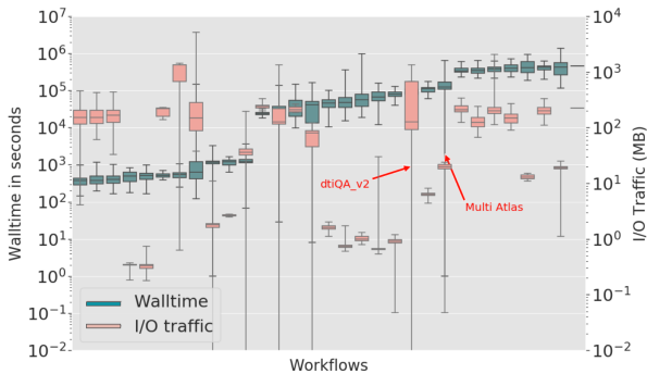
Figure 2. Range of walltime (in red) and I/O traffic (in green) for 31 representative neuroscience workflows running on the ACCRE cluster between 2013 and 2016. The workflows are sorted by their median walltime. Vertical lines show the intervals between the minimum walltimes and the maximum walltimes, bins show the 10th to 90th percentiles, and the horizontal lines highlight the medians.
