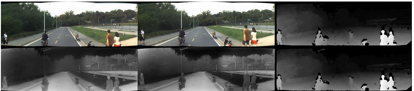
Fig. 7. The output pixel-wisely aligned wide-view RGB, thermal and disparity images at a certain time instance. Left column: the output of the top camera array. Middle column: the output of the bottom camera array. Right column: the top one is the disparity map obtained only based on the RGB image, and the bottom one is obtained based on the RGB and thermal frames.
