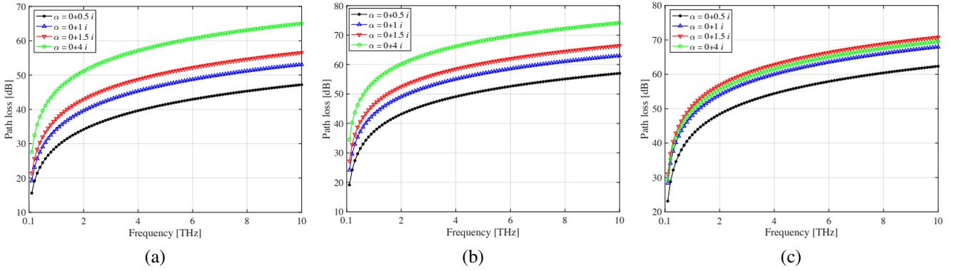
Fig. 6. Attenuation behavior versus the frequency in case of  $Z_{load} = 1/(j\omega C)$  with  $C = 50pF$ , and for different values of  $\alpha$ , in case of different metasurface length [m] set to (a)  $r = 0.01$ , (b)  $r = 0.1$ , and (c)  $r = 0.3$ .
