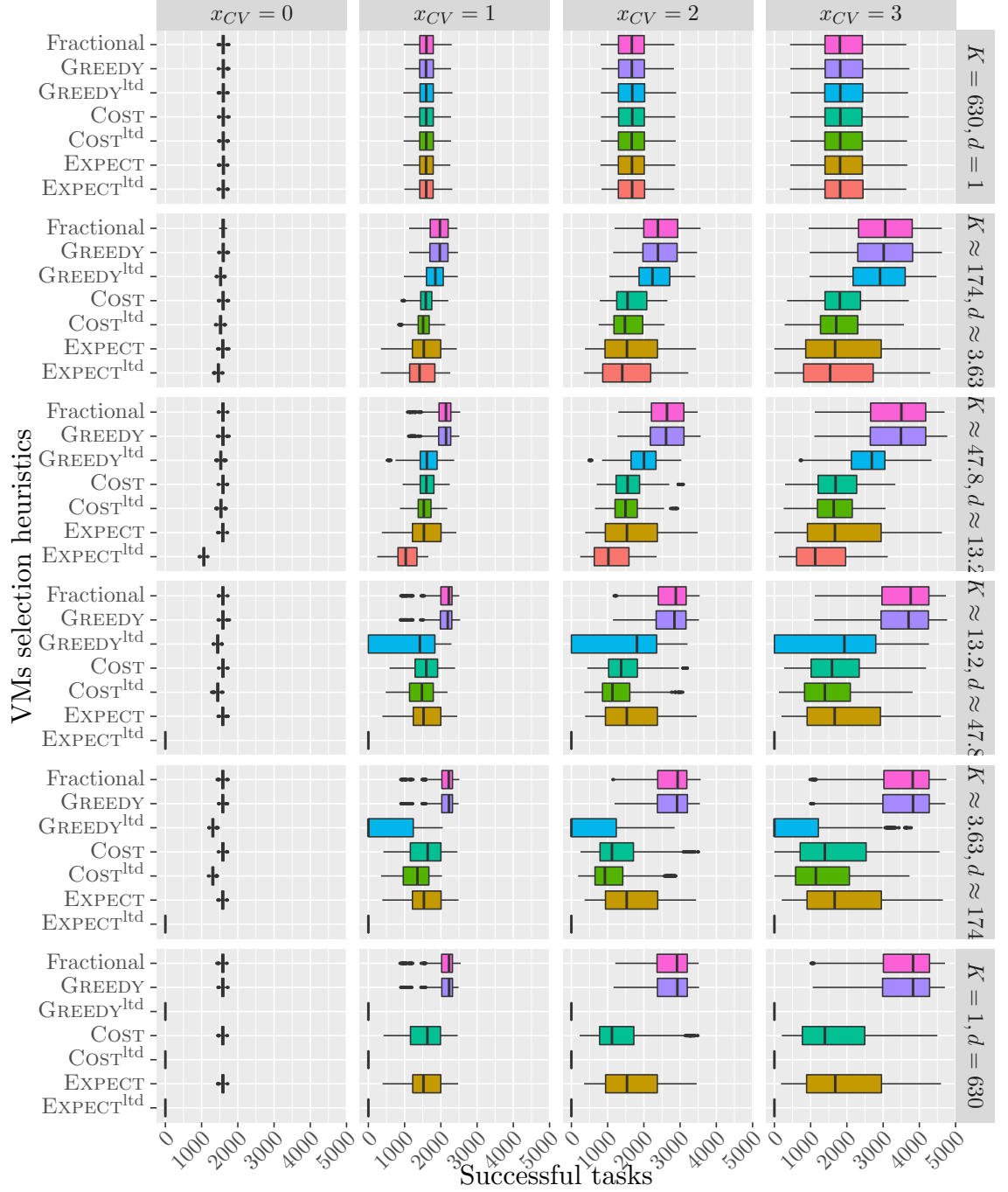
Figure 6: Number of successfully executed tasks of different methods to choose VMs when interrupting tasks with heuristic OPTRATIO. Each of the 100 platforms is generated with m_j = 10 , M = 60 , c_j = s_j and is used 10 times with b = 630 . The values for d and K follows a geometric progression between 1 and 630. Execution times follow either a lognormal distribution with x_{CV} = 0, 1, 2, 3 .
