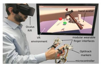
Fig. 10. Experimental setup. Subjects were asked to interact with the virtual environment while wearing two wearable cutaneous devices, one on the thumb and one on the index finger. The virtual environment is composed of seven different objects lying on a table. Interaction forces in the virtual environment are provided to the user by the cutaneous device as indicated in Sec. II.
