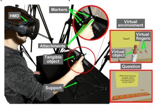
Figure 2: Setup for the experiment. Insets show the virtual environment during the task.
