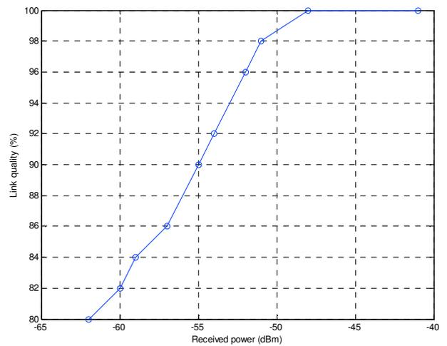
Fig. 7. Link quality as function of received power
