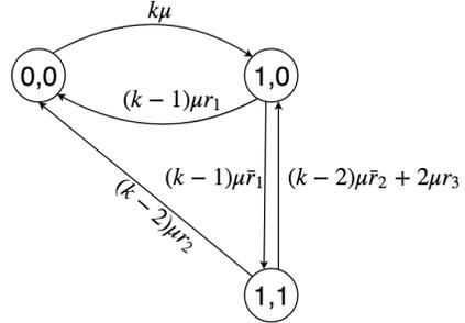
Fig. 1: CTMC for a system with at least three links and buffer size one for each link.  $k$  is the number of links,  $\mu$  is the rate of entanglement generation, and  $r_1$ ,  $r_2$ , and  $r_3$  are parameters that specify the scheduling policy.
