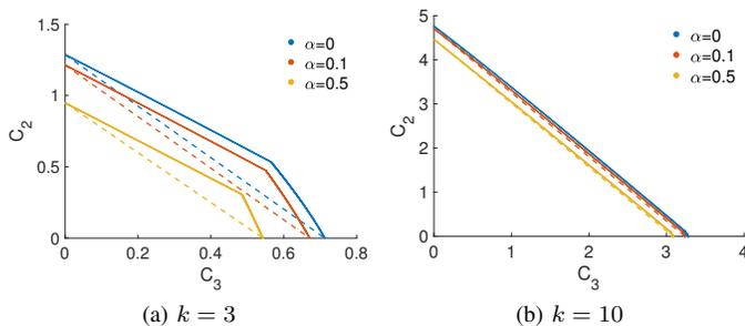
Fig. 9: Capacity region for a system of buffer size two and varying number of links  $k$ , decoherence rates  $\alpha$ , and entanglement generation rate  $\mu = 1$ . The solid lines are the upper boundaries of the capacity region, and the dashed are TDM lines.
