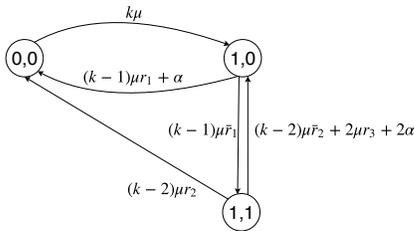
Fig. 7: CTMC for a system with at least three links and buffer size one.  $k$  is the number of links,  $\mu$  is the rate of entanglement generation,  $\alpha$  is the decoherence rate, and  $r_1, r_2, r_3$  are parameters that specify the scheduling policy.
