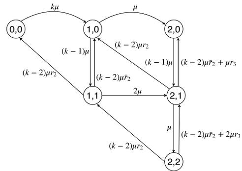
Fig. 4: CTMC for a system with at least three links and buffer size two for each link.  $k$  is the number of links,  $\mu$  is the rate of entanglement generation, and  $r_2$  and  $r_3$  are parameters that specify the scheduling policy.
