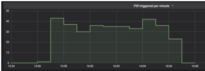
Fig. 8. Chart of PIR signal values that display one sitting session
