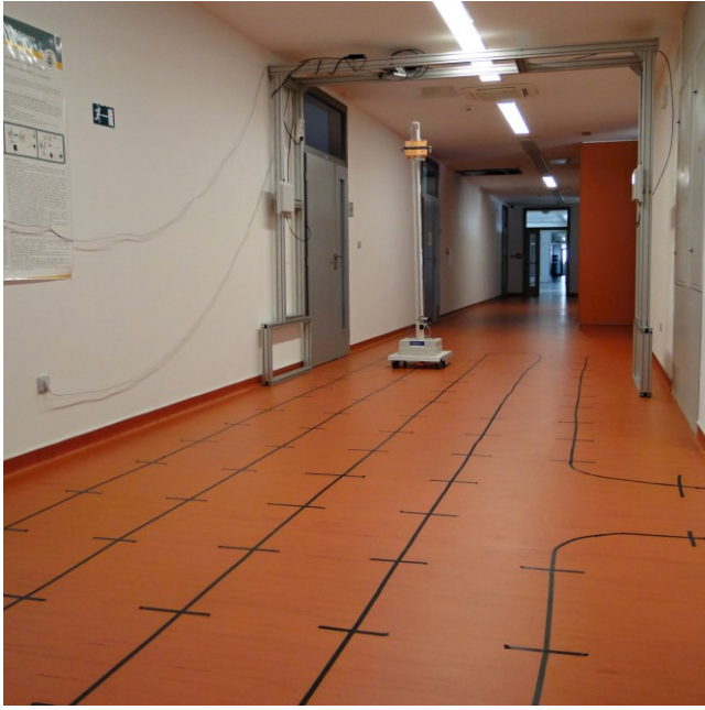
Fig. 10. Autonomous system for measuring of RSSI during the test.
