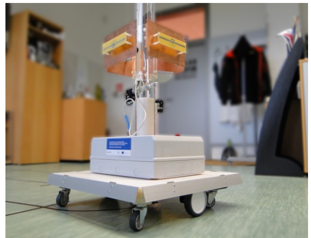
Fig. 5. Autonomous system for measuring of RSSI – UHF RFID tags (Etalons).
