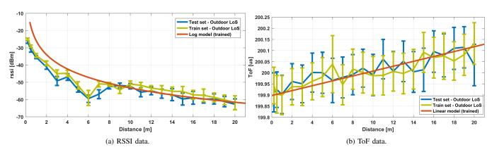
Fig. 2: Acquired data: RSSI values (a) and Time of flight (b), plotted with respect to nodes distance in the Outdoor LoS condition. The mean value over 1000 ToF samples is reported, error bars are one standard deviation high. The two colors depict the train and test dataset. The fitted model is in red.
