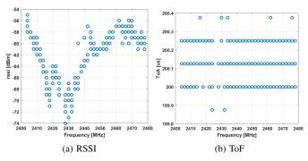
Fig. 4: Effect of channel hopping on raw (not averaged) RSSI and ToF data. Each figure contains 1000 data points, then each circle may represent multiple overlapped points.
