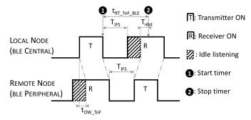
Fig. 1: Connection event representation. The One-Way propagation time  $t_{OW\_ToF}$  is exaggerated to highlight the details of the measurement. Figure not to scale.
