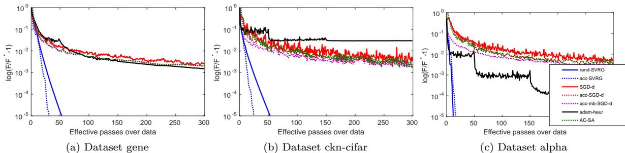
Figure 1: Optimization curves without perturbations when using the logistic loss and the parameter  $\lambda = 1/10n$ . We plot the value of the objective function on a logarithmic scale as a function of the effective passes over the data (see main text for details). Best seen in color by zooming on a computer screen. Note that the method Adam is not converging.
