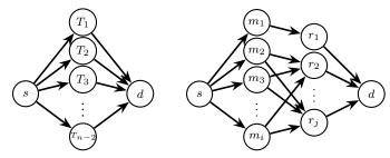
Fig. 3: Example of simple (left) and single-stage (right) MapReduce workflows with i map tasks and j reduce tasks.
