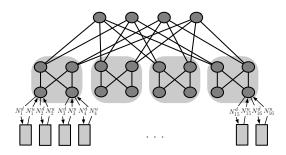
Fig. 2: Modeling data center communications with Network machines for a 4-Fat Tree with 16 (racks of) servers.
