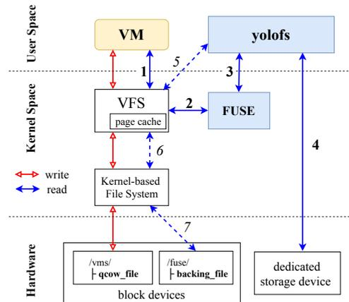
Fig. 7: yoloofs read/write data flow
