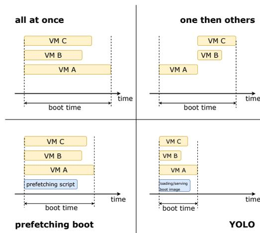
Fig. 8: Four investigated boot policies. Each block represents the time it takes to finish. *Prefetching boot* performs prefetching in a parallel fashion to leverage gaps during the booting process of a VMs for faster loading. *YOLO* loads and serves boot images whenever VMs need to access the mandatory data.
