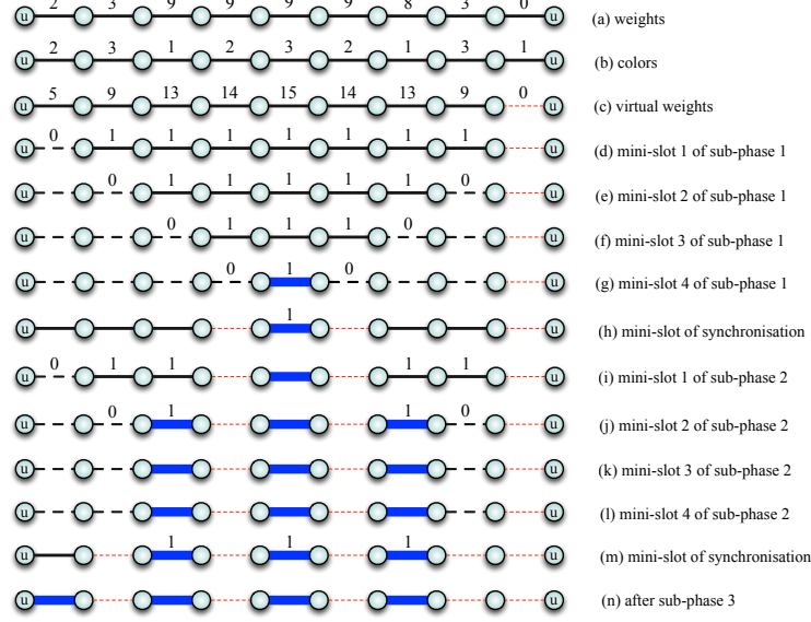
Fig. 6 Output of \text{AlgoLog} for a cycle composed of 9 links for d = 0 , C = 3 , K = 5 , L = 4 , W = 15 , and T = 4 . Active links are indicated with thick bold blue lines, inactive links with thin dashed red lines, undetermined links with thin black lines, and potentially inactive links with dotted black lines.
