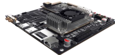
Nvidia GTX Jetson TX1 Generation Maxwell
