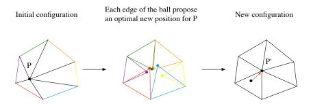
Fig. 7 Laplacian smoothing in two dimensions. Each element of the ball of considered vertex  $P_i$  suggests an optimal position for  $P_i$ . The resulting new optimal position for  $P_i$  is computed as a weighted average of all these proposed locations.
