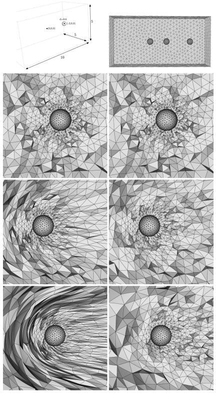
Fig. 12 Case of the moving sphere inside a  $P^2$  mesh. First line, description of the sphere and description of the three considered positions of the moving sphere: the sphere is moving from right to left. And then, from top to bottom, zoom in the vicinity of the sphere for each position. Left, without mesh optimization operators. Right, with mesh optimization operators.
