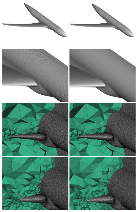
**Fig. 11** NASA Common Research Model aircraft meshes. From top to bottom, surface, coarse and fine meshes. From right to left,  $P^1$  and  $P^2$  meshes.  $P^2$  meshes are generated with Algorithm 1 using a cubic reconstruction.
