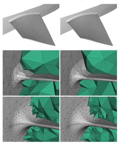
**Fig. 10** NASA RO37 rotor turbomachine meshes. From top to bottom, surface, coarse and fine meshes. From right to left,  $P^1$  and  $P^2$  meshes.  $P^2$  meshes are generated with Algorithm 1 using a cubic reconstruction.
