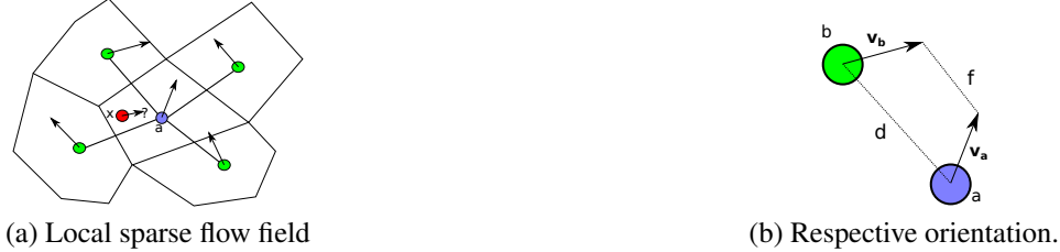
Fig. 2. Interpolation of flow vector at x (in red) according to the central flow vector (in purple) and the neighbouring flow vectors (in green). The purple and green points are the centers of their respective superpixels delineated by black lines.
