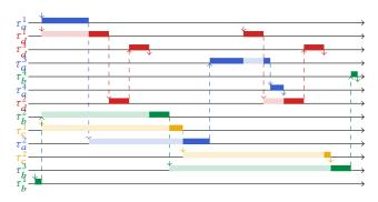
Figure 1: A system with four task chains. Task priorities are decreasing from top to bottom.
