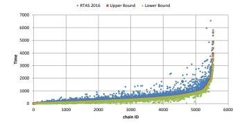
Figure 2: Latency bounds for periodic and sporadic synchronous chains.
