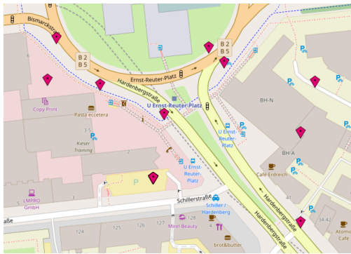
Fig. 7. T-Mobile BS configuration in Berlin.
