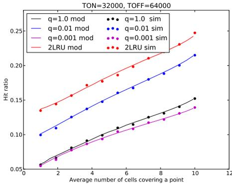
Fig. 5. Trefoil: results for the *lazy* update rule and an ON-OFF request process with  $\mathbb{E}[T_f^{ON}] = 3.2 \cdot 10^4$  and  $\mathbb{E}[T_f^{OFF}] = 6.4 \cdot 10^4$ . The cell request rate for the most popular content is  $\Lambda = 1.3$ .
