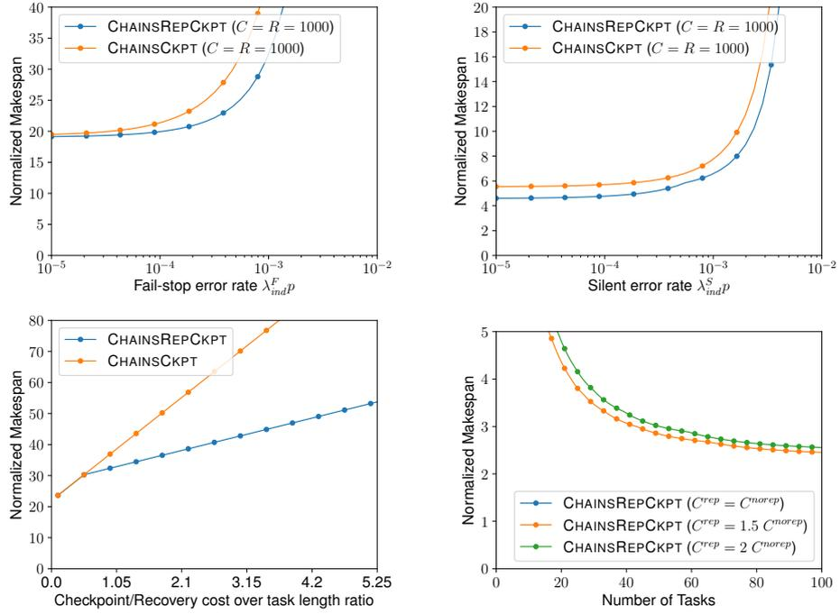
Figure 10: Impact of fail-stop error rate  $\lambda_{ind}^F p$  (left), checkpoint cost (middle) and ratio  $\alpha$  between the checkpointing cost for replicated task  $C_i^{rep}$  over non-replicated tasks  $C_i^{norep}$  (right) for the UNIFORM distribution.
