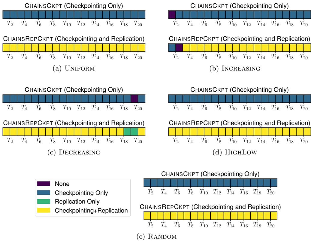
Figure 8: Optimal solutions obtained with the CHAINSCKPT algorithm (top) and the CHAINSCKPT+Replication algorithm (bottom) for the five work distributions.
