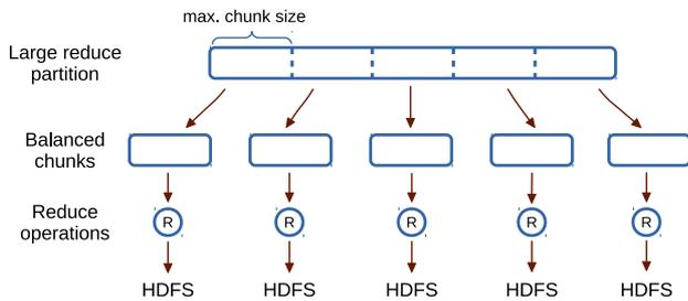
Figure 6: Load balancing mode in Flame-MR
